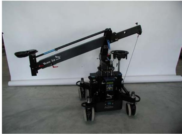
The Jib cable can be used instead of the Jib A-Round-Kit. It is mounted to the back outrigger and on two wheel arms.
