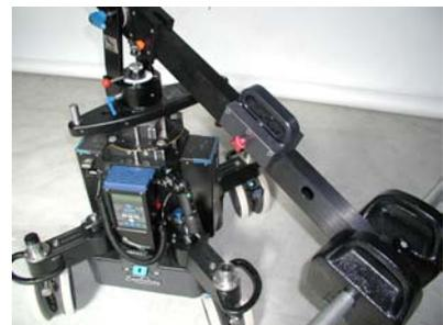
The Euroadapter gets levelled by turning the blue levelling rod.
