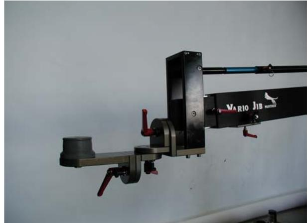
1. The Multi Rig is attached under the front bearing of the Vario Jib.
