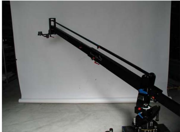
The Extension is mounted between the telescopic tube and the end-section. Take off (unscrew) the blue leveling rod and extend it with the extension rod. The second counterweight rod is put into the second hole of the back outrigger and loaded.
